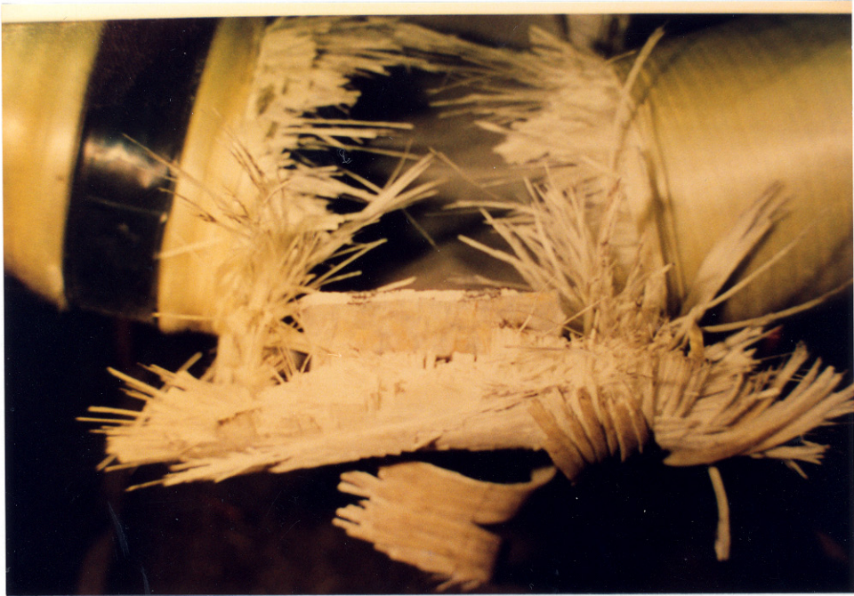
12. Closeup View of the Rupture Location
